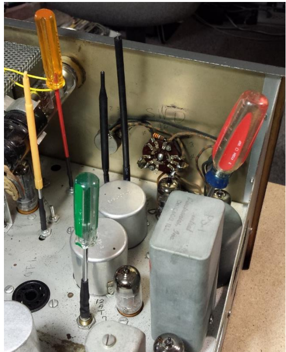
Figure 5. Alignment screwdrivers held up by heat shrink sleeves.
