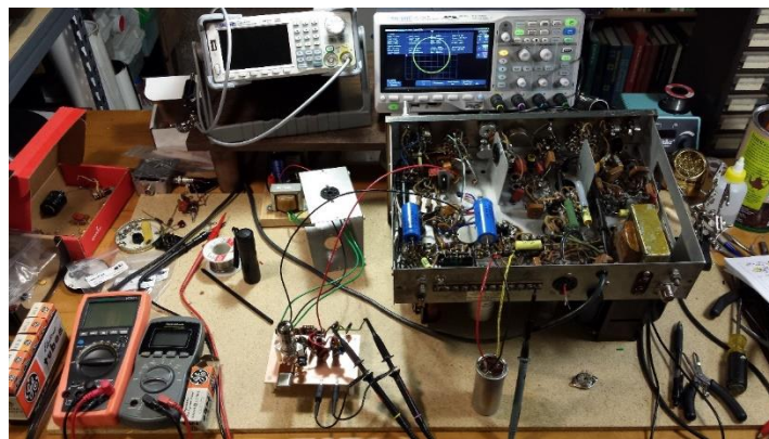
Figure 2. External 9 MHz oscillator and 90-degree RF phase shift display.
